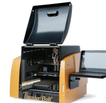
The ThunderBolt® is an innovative 2-plate, fully automated, open platform that is compact and cost efficient. The user friendly and flexible software is capable of programming a broad range of protocols. The ThunderBolt® is available for both ELISA and Chemiluminescent (CLIA) applications.
